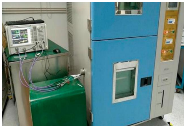
Fig. 4: Experimental setup for temperature and humidity cycling test
